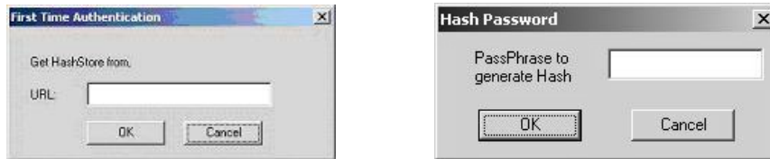
Fig. 3. At left, the client requests URL entry for hashstore; at right, the client requests the passphrase to generate the HMAC.
