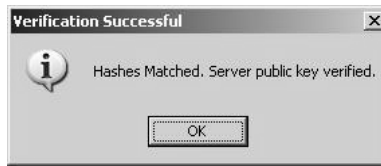
Fig. 4. If the retrieved HMAC matches the public key the server sent, then the server has been authenticated.
