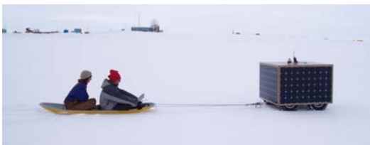
Fig. 6 Cool Robot pulling a sled on the skiway during traction tests.
