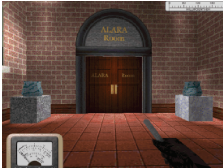
Sim Room for Simulation #2. Trainee must use Ludlum radiation meter to check anteroom for background radiation levels. Note meter readout in left lower area of the screen. Dosimeter reading is in the right upper corner.
